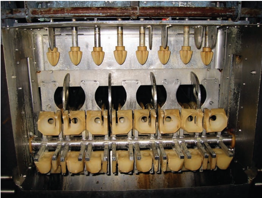
FIGURE 4.6 “Brown” process. A battery of eight juice squeezers waiting for fruits.
