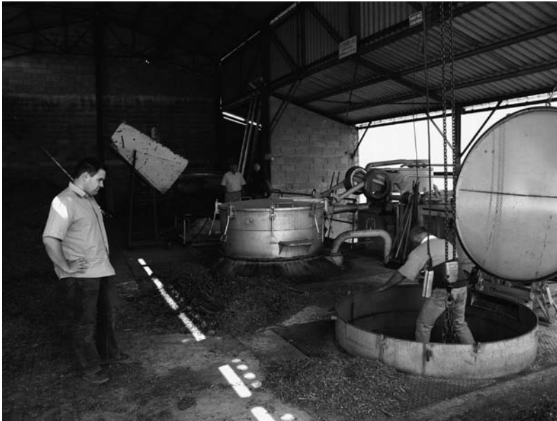
FIGURE 4.14 Loading a kettle and pressing by concreted tractor wheel.
