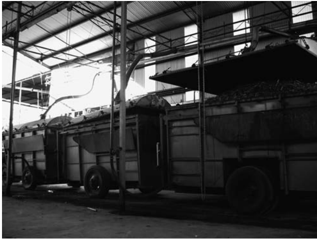
FIGURE 4.21 A battery of containers to be distilled, one opened to show the biomass.
