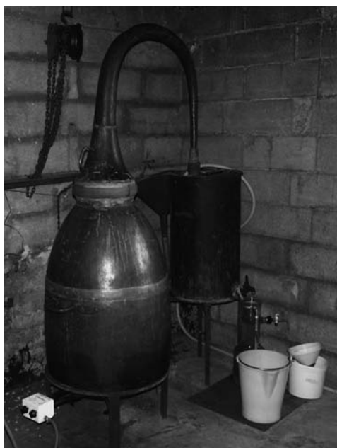
FIGURE 4.9 Old distillation apparatus modernized by electric heating.
