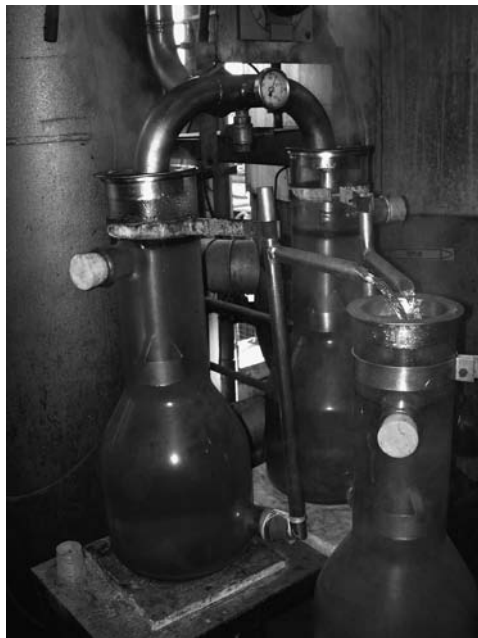
FIGURE 4.19 Orris distillation, Florentine flask at nearly 98°C.
